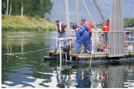
Figure 2. U.S. Geological Survey personnel collecting a 3.7-meter-long vibracore sample of riverbed sediments in the Kootenai River, Idaho. (from Barton, 2004)
