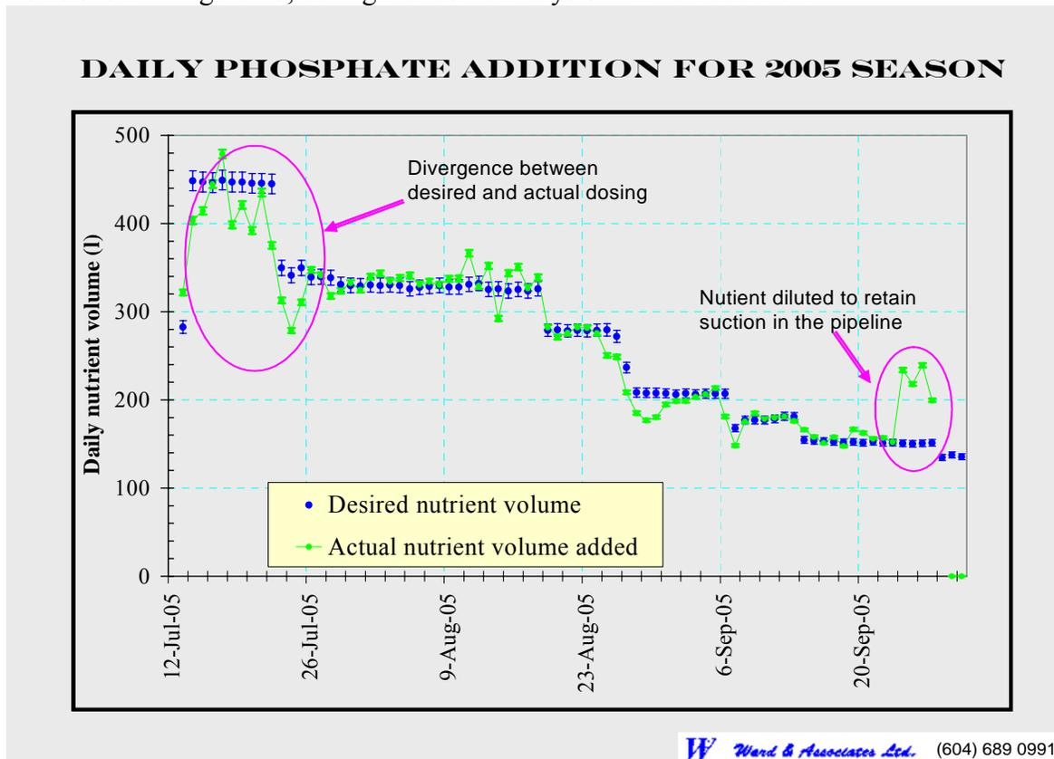
**Figure 16. Daily Volume of 10-34-0 Nutrient Dosed, Compared with Desired Volume to Achieve Target Concentration of P in the River.**
