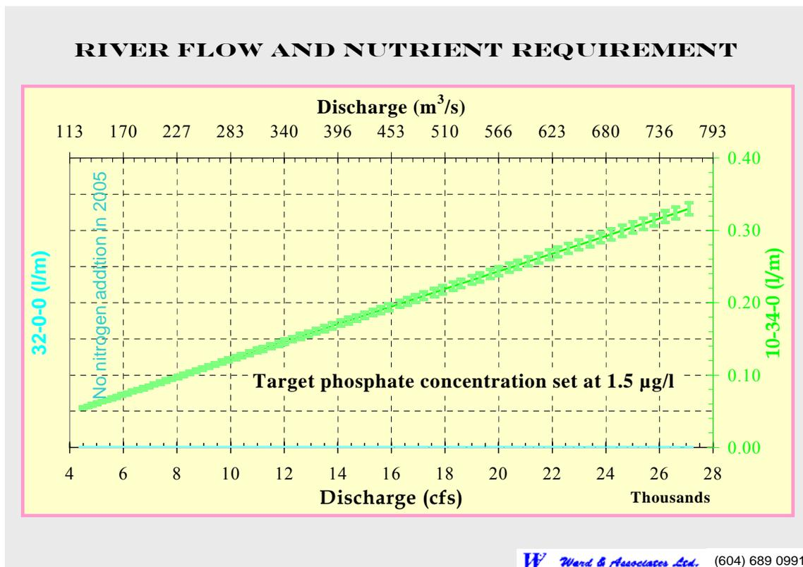
**Figure 14. Flow rate of 10-34-0 Needed to Create Desired Concentration of P in the River**
