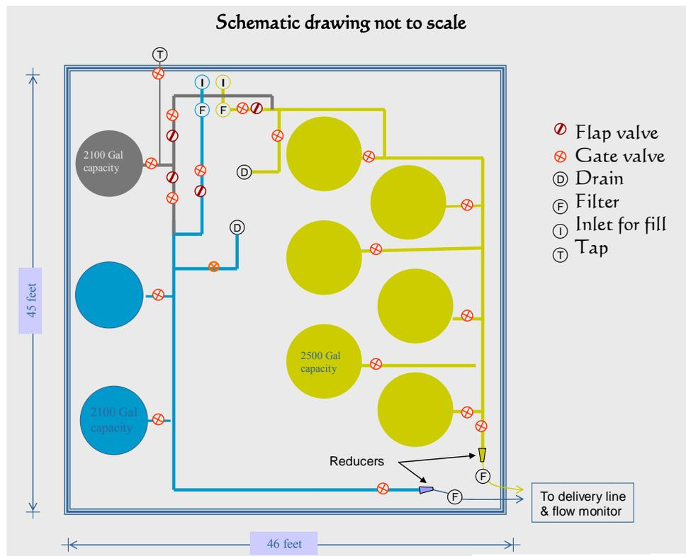
**Figure 4. Schematic of Tank Farm Showing Configuration of Manifolds**
